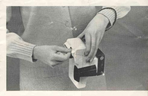
Here's an important reminder: This is the only correct way to hold the camera when you develop the picture.
