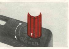
Picture too light or too dark? To darken the next picture of the same subject in the same lighting conditions, turn the silver pointer on the red knob toward DARKEN; to lighten the picture, turn it away from DARKEN. For a small change, move the pointer one mark; for a bigger change, move it two marks.
