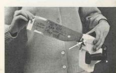
Tear off the paper along the dotted line: Start at the edge near the blue button (arrow). Tear up and toward you. You're ready for picture No. 1.
