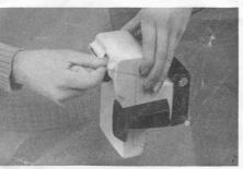
Push the blue button with your RIGHT thumb until you hear a click: Keep the button pushed in and grip the film firmly with your right thumb and forefinger.
