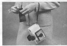
**Peel off the print:** Insert a fingernail in the curved slot (arrow).
